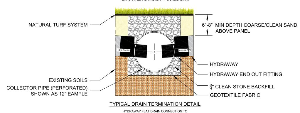
PERFORATED PERIMETER PIPE UNDERDRAIN
