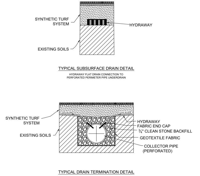
HYDRAWAY FLAT DRAIN CONNECTION TO PERFORATED PERIMETER PIPE UNDERDRAIN
