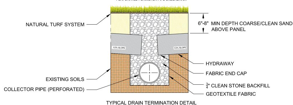
HYDRAWAY FLAT DRAIN CONNECTION TO PERFORATED PERIMETER PIPE UNDERDRAIN
